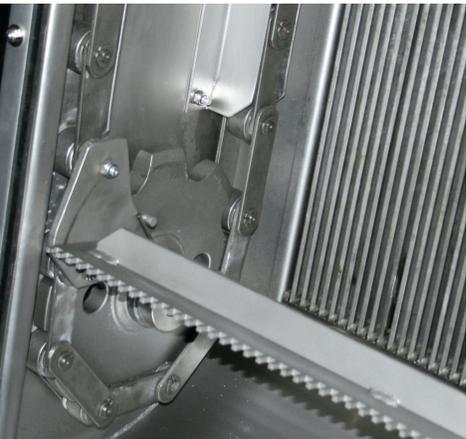
The Kusters Water ProTechtor® Multi-Rake Bar Screen combines fine or coarse screening with high solids capture rates. Its robust construction and overload feature ensure reliable operation.
